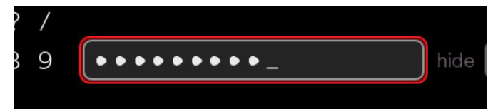
Same text field with user focus. By default the passwords masks (with bullets) as its being typed, but this can be unmasked by unchecking the tick box on the right. Note the characters are further apart in the password field.
